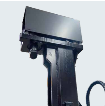
Improved design with built-in cabling and larger bending radius for hydraulic hose between pocket and end-post.
