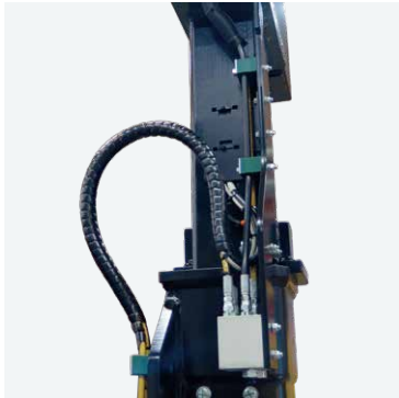
Improved design with built-in cabling and larger bending radius for hydraulic hose between pocket and end-post.
